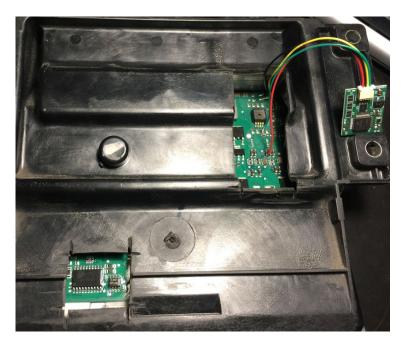
We solder EMU as on picture. Not need to solder any jumpers on EMU. We read 95160 EEprom and first 2 lines (adres 0-1F we fill value 00).
