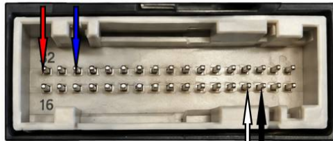
T32 pinout (view from rear, wiring side)
