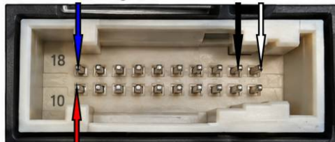
T18 pinout (view from rear, wiring side)
