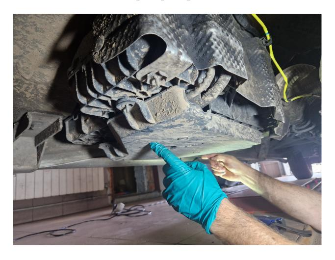
Disconnect Pump connector as on picture:
