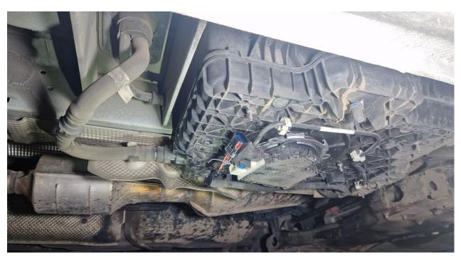
Disconnect NOX2 sensor as on picture
