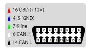
Blue wire from the car we connect to PIN 14 UHDS OBD connector (CAN L) Red wire from the car we connect to PIN 6 UHDS OBD connector (CAN H)  $^{\circ}$
